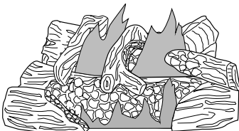
Figure 55 - Typical Flame Pattern
