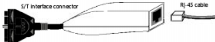
Connecting the S/T interface connector and RJ-45 cable
