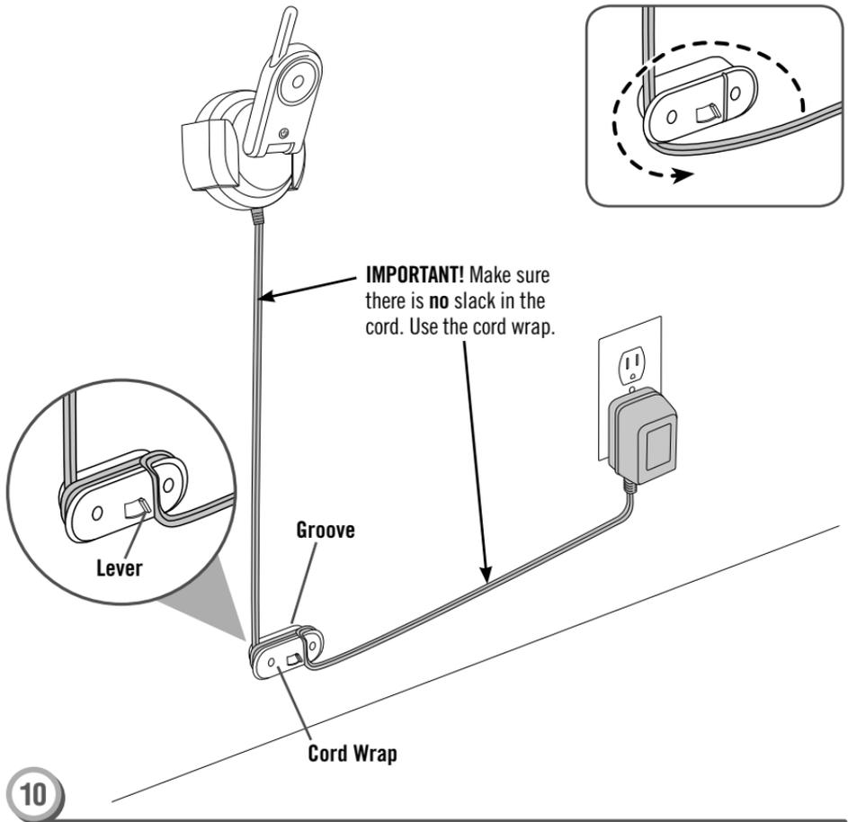
**IMPORTANT!** Make sure the cord is taught between the camera docking station and cord wrap. Excess cord can form loops or extend into the crib and present a strangulation hazard.
