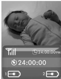
**Notes:** The number next to the on-screen battery indicator corresponds to the number on the back of the parent unit and camera. Both battery indicators are only visible when the parent unit is in a vertical view. When the parent unit is in a horizontal view, only the parent unit's battery indicator displays.
