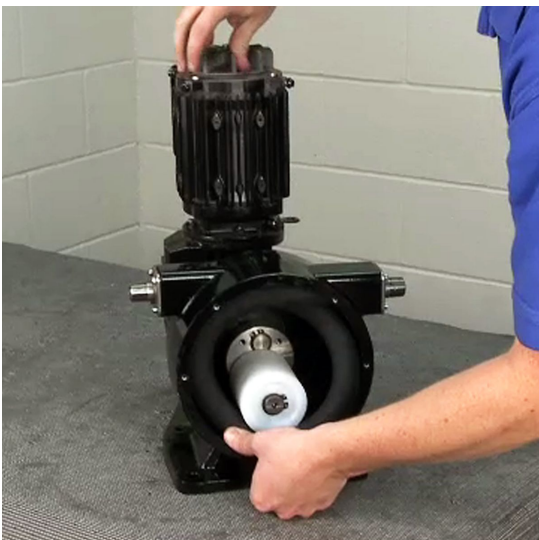
Figure 9 Roller in 6 O'Clock Position
