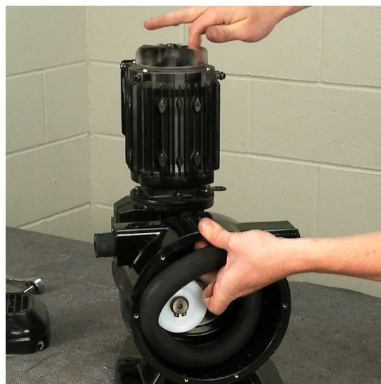
Figure 4 Roller in 9 O'Clock Position
