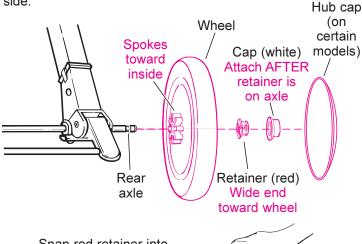
Snap red retainer into axle groove. Then snap cap over red retainer as shown. Be sure cap is snapped securely over red retainer.
