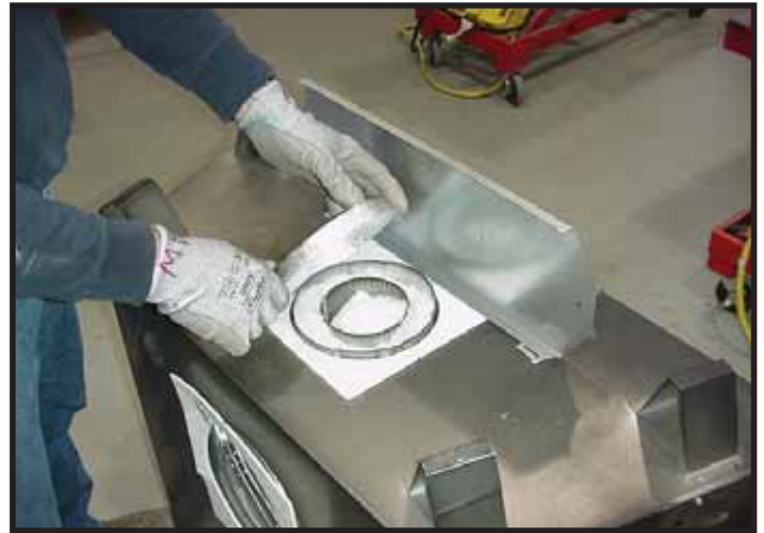
Figure 9.4 Remove the seal cap.
