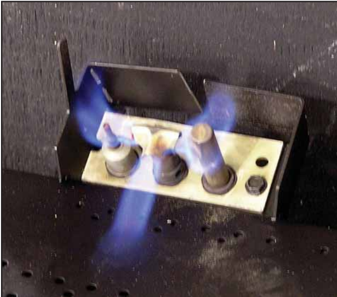
Figure 3.2 Standing Pilot Flame Patterns
