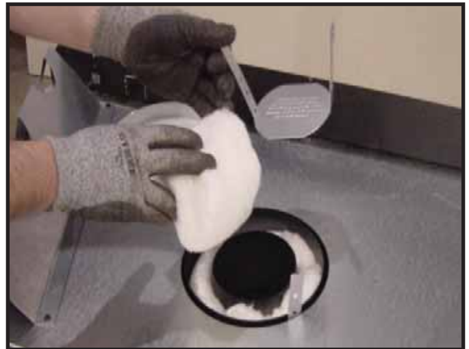
Figure 9.4 Remove the insulation basket and white insulation from the center vent pipe.
