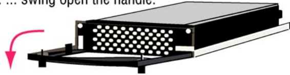
Fig. 41. Handle on mounted hard disk.
