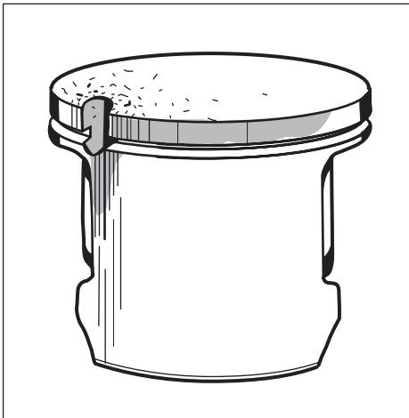
The guide pin for the piston ring has been pushed up through the top of piston.
